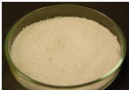
Figure 27: Sample of magnesium sulphate powder - one of the thermochemical materials under investigation.
