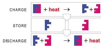
Figure 26: The principle of thermochemical heat storage: heat is used to separate a chemical compound into its component parts. The components can then be stored for long periods with practically no heat loss. When the components are reunited, a chemical reaction occurs and heat is produced. (Source: ECN, The Netherlands)
