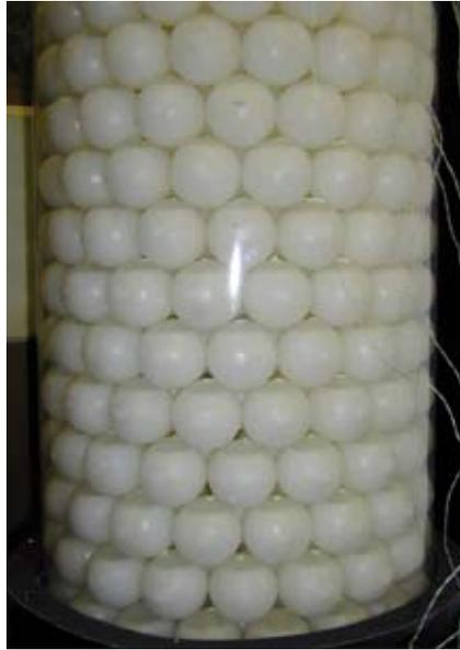
Figure 25: An experimental latent heat storage with macro encapsulated PCM (paraffin). (Source: Ciril Arkar, University of Ljubljana, Slovenia)
