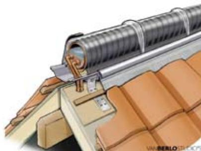
Figure 28: Example: A solar thermal roof-ridge collector is a "hidden" installation, which is already used in a few EU countries. It provides solar heat and also acts as a "standard" roof ridge. It has been developed primarily as an architectural solution to the integration of solar active roof elements, which will not impede subsequent roof alterations, such as the installation of a dormer window.
