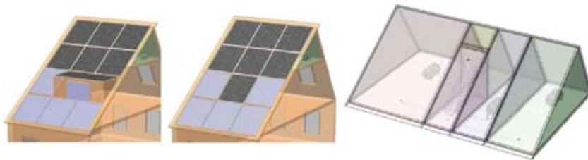
Figure 31: Modular roof elements for solar thermal and solar electrical panels (with or without a window) in combination with heat storage in the attic. (Source: ECN, The Netherlands)
