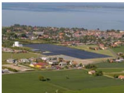
Figure 21: Marstal (DK) 12.9 MW<sub>th</sub> capacity (18,365 m<sup>2</sup> collector area), integrated into the local district heating system. The world's largest solar thermal plant provides 30% of the total heat demand of a Danish island. (Source: Arcon Solvarme A/S, Denmark)
