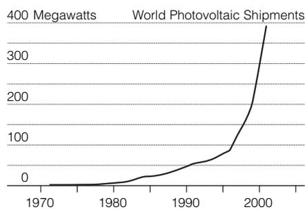
Fig. 15a The dramatic increase in world photovoltaic module shipments. It surpassed 500 MW<sub>p</sub> in 2002. Data source: Paul Maycock.
